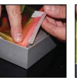
Step 1 Insert corner A Turn edge of graphic so silicon welt is perpendicular to face of graphic. Insert narrow side of welt with fabric to outside into the channel. Repeat for other side of this corner
